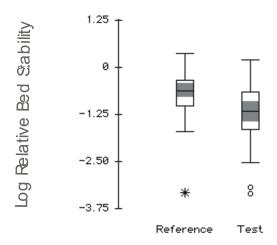
Figure 7. Box plots of log relative bed stability in reference sites vs. test sites; p = 0.0025 (Mann-Whitney U).
