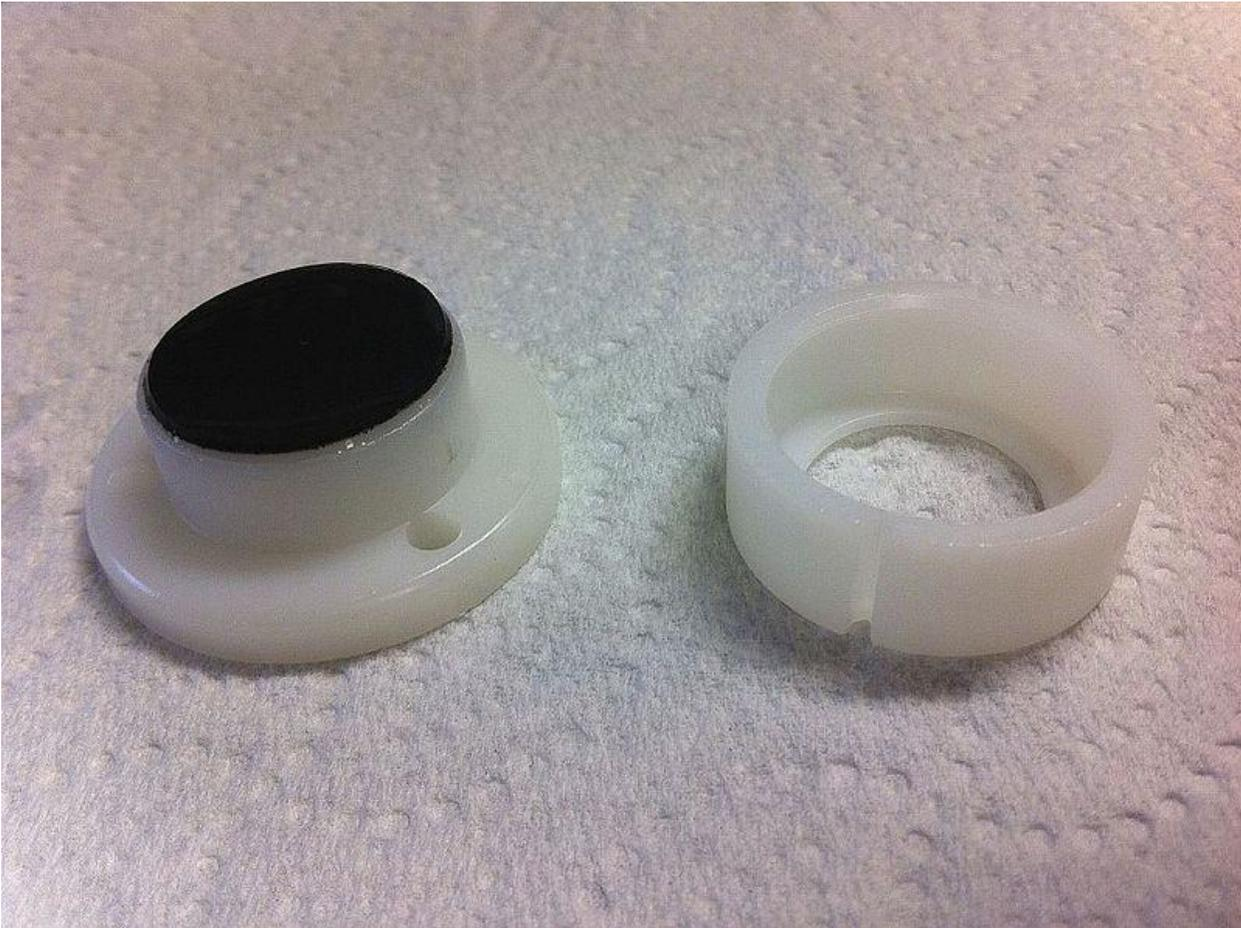
Figure 7. CLAM passive sampler
