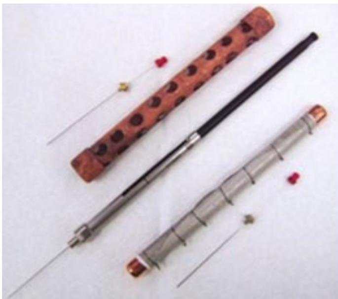
Figure 6. Organic Diffusion Gradients in thin films (o-DGT) device piston and cap
