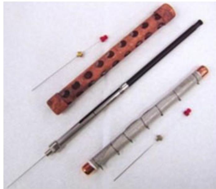
Figure 6. Organic Diffusion Gradients in thin films (o-DGT) device piston and cap
