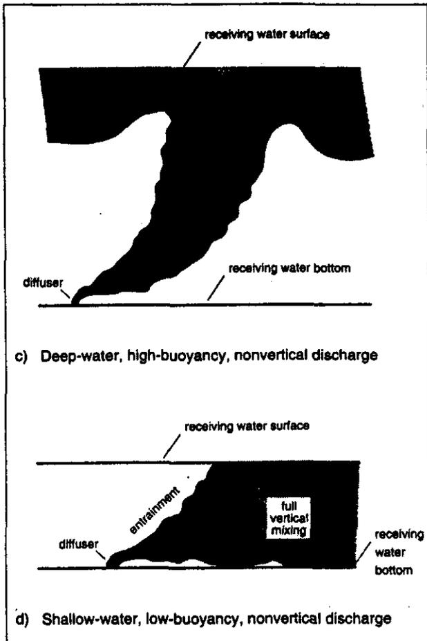
Figure 4-2. Example of Discharge-Induced Mixing [7]
