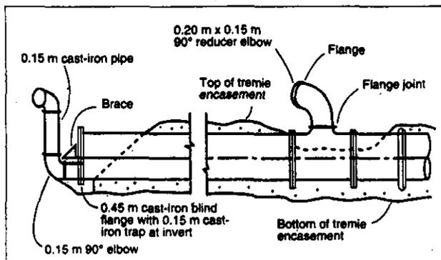
Figure 4-1. A Typical Diffuser Section [17]
