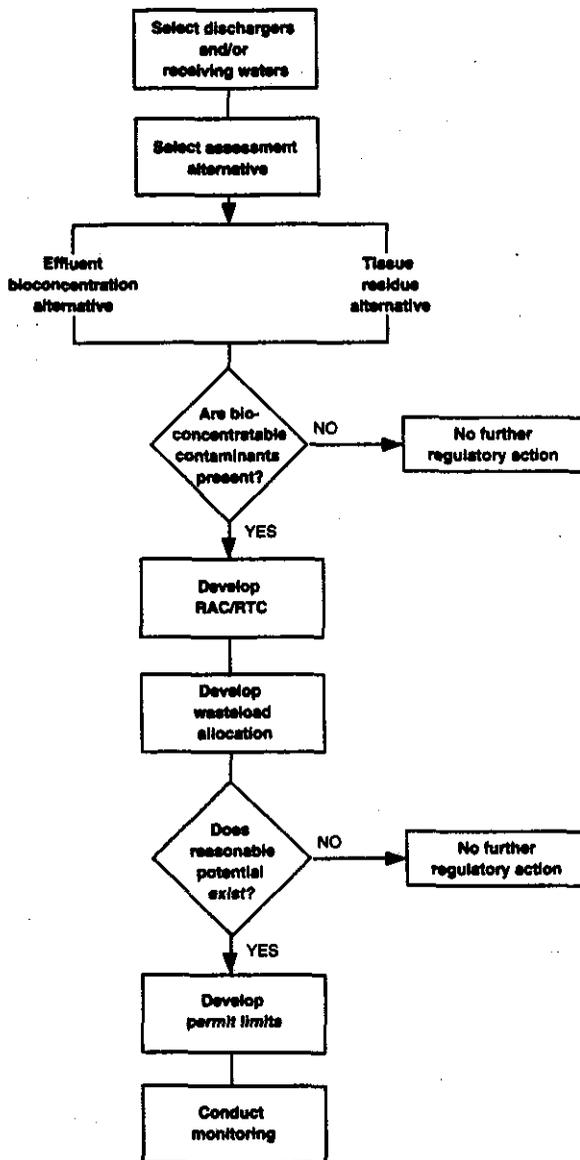
Figure 3-6. Procedure for Assessment and Control of Bioconcentratable Contaminants in Surface Waters
