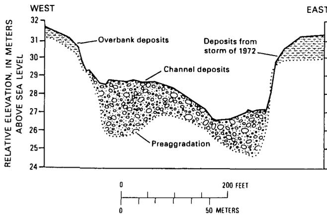
FIGURE 10. — Recent changes in the geometry of Redwood Creek at the mouth of Tom McDonald Creek. Preaggradation configuration was estimated from reports of local forest workers and road construction records. Configuration in 1972 is from ground surveys.
