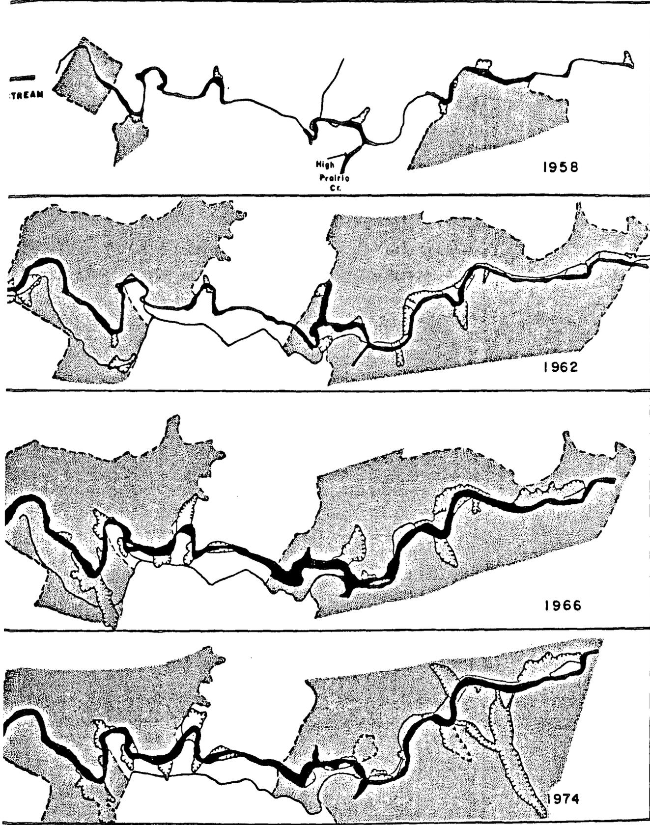
FIGURE 20. Sketch maps of a part of the Redwood Creek channel between Snow Camp Creek and State Highway 289 traced from aerial photographs. Approximate scale 1:12,000. Stream channels are shown in black, streamside logging by shaded areas, roads by thin black lines, active landslides by hachured lines, healing landslides by dashed hachured lines, and flat-topped berms bearing live or upright dead vegetation by open circle patterns.
