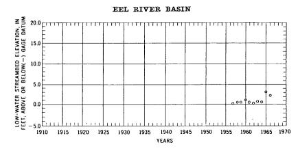
Gaging-station number: 11-4722. Gaging-station name: Outlet Creek near Longvale, Calif. Elevation of gaging-station datum, in feet, above msl: 1,020. Notable flood peaks: 26,500 cfs Feb. 8, 1960; 77,900 cfs Dec. 22, 1964.
