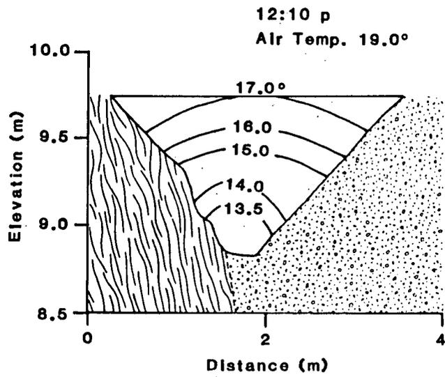
Figure 30. Bulges in temperature profiles indicate cold water contribution to pools. In contrast, cold pools formed by depth alone have horizontal isotherms.
