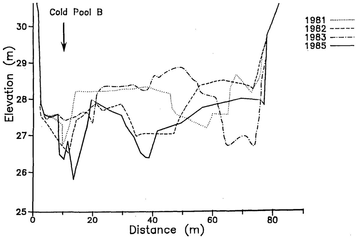
Figure 20. Mainstem Cross Section K-L shows that the channel shifts position annually. The Tall Trees Grove Cold Pools are located adjacent to the left bank. Note that in years when the low flow channel is in the middle or right side of the channel, a pool forms on the left bank (Redwood National Park, unpublished data).
