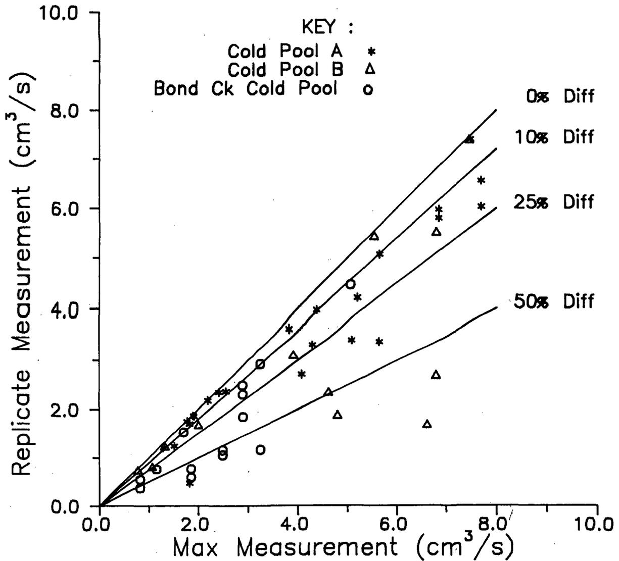
Figure 12. Plot of replicate seepage meter measurements against the highest measured seepage rate at the same meter. The solid lines represent the percent difference between successive measurements.
