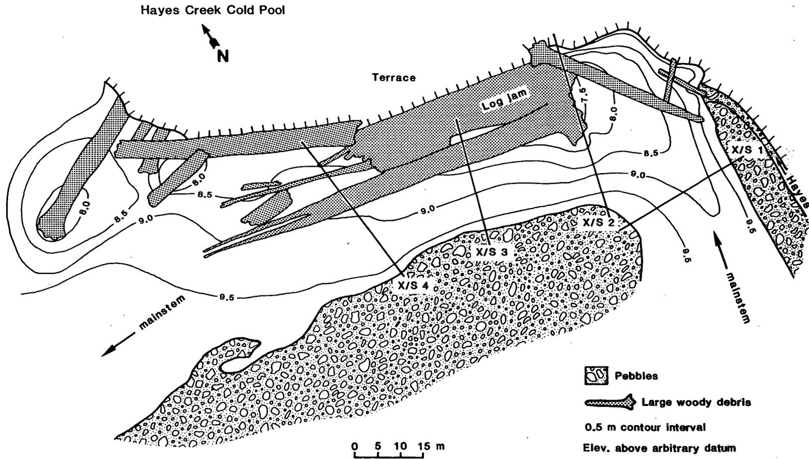
Figure 27. Topographic map of the Hayes Creek summer pool showing cross section locations. The pool was located on the right bank downstream of Hayes Creek.
