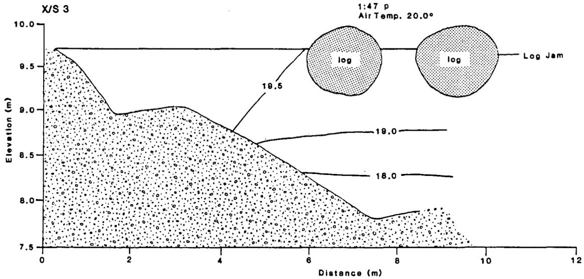
Figure 28. Pool water was stratified under the log jam (Cross Section 3). However, temperature profiles immediately upstream and downstream of the log jam were uniform in temperature.
