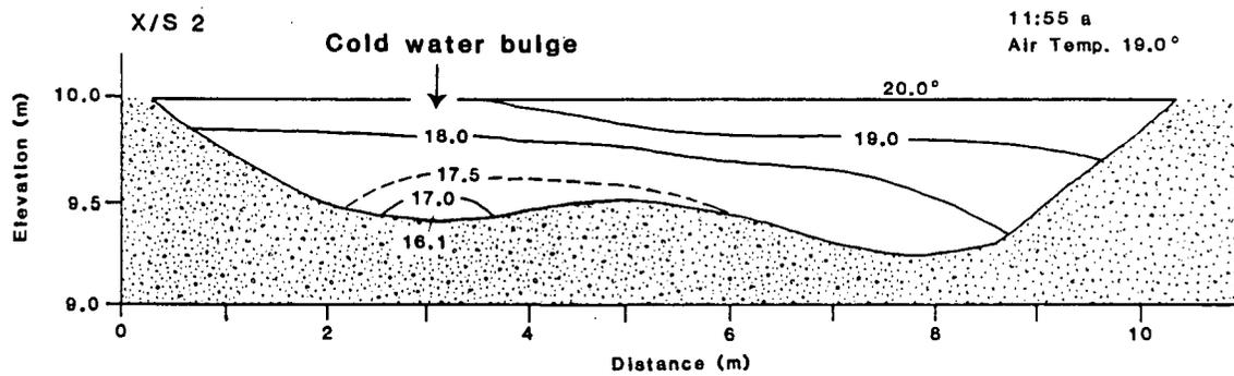
Figure 22. Temperature profile of Cross Section 2 in the Bond Creek Cold Pool shows a small cold water bulge on the left side of the pool.
