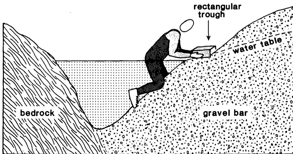
Figure 8. A 17-cm wide rectangular trough was inserted into the gravel bar above the pool surface to measure inflow volumetrically.
