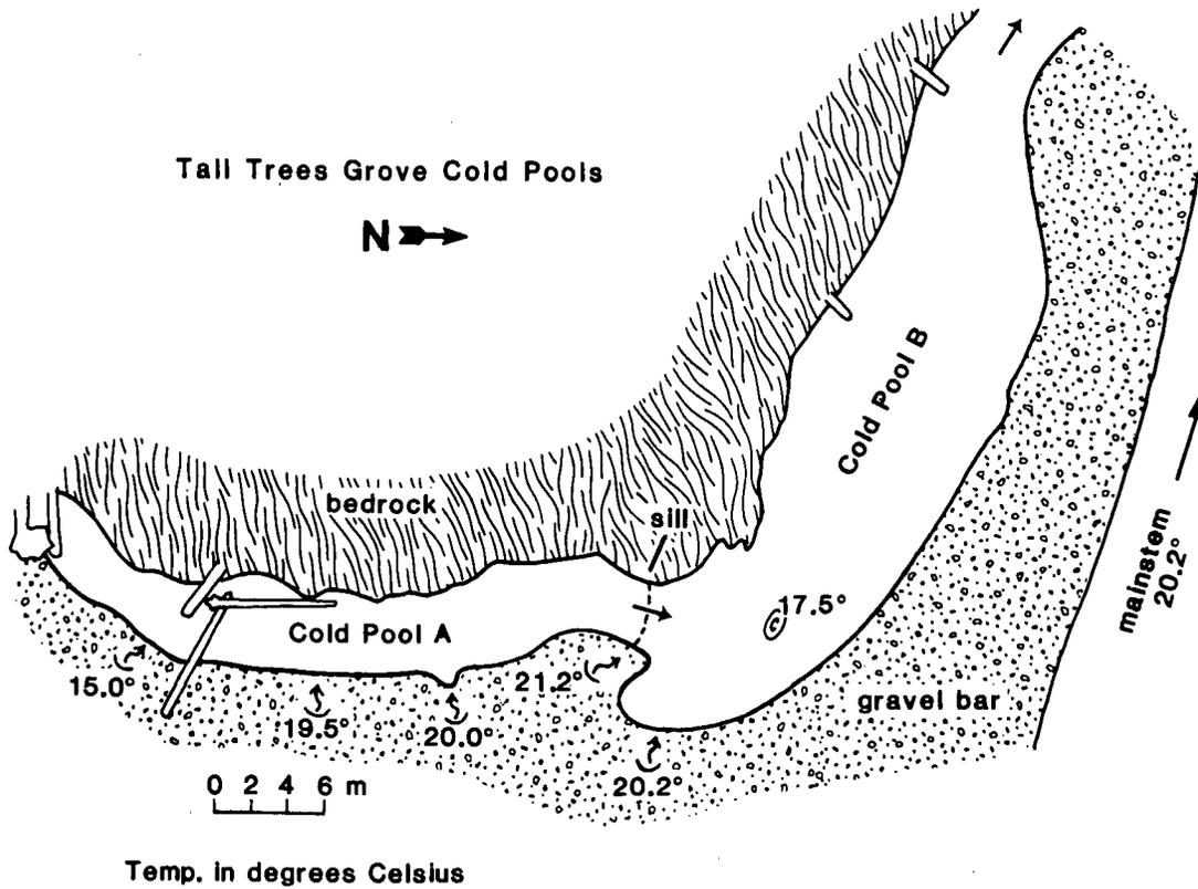
Figure 19. Temperature of near surface intergravel flow increased with distance from the hillslope in the Tall Trees Grove Cold Pools. Temperatures were measured on August 1, 1985.
