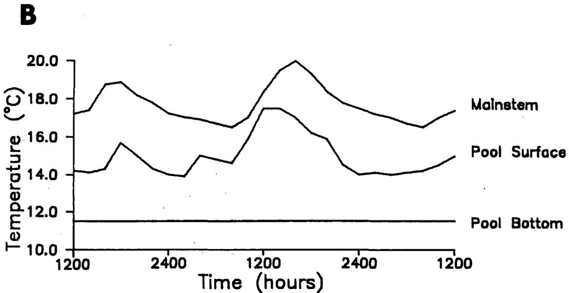
Figure 17. Thermographs were located at the head of Cold Pool A and in the mainstem (A). Water temperatures recorded over a two day period in August in Cold Pool A showed that cold pool water never exceeded mainstem temperatures (B).
