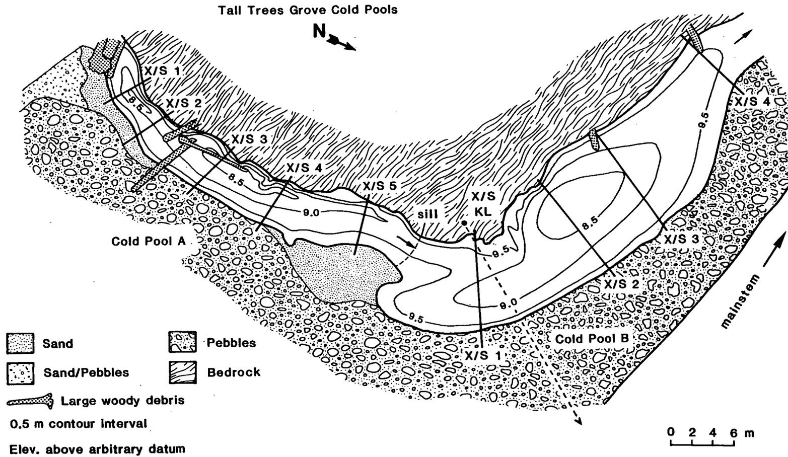
Figure 15. Topographic map of Cold Pool A and B showing cross section locations. The pools were located on the left bank of the channel and a shallow sill separated the cold pools.
