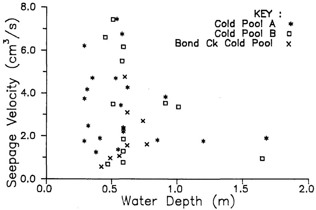
Figure 13. Plot of seepage rate against water depth at seepage meters.
