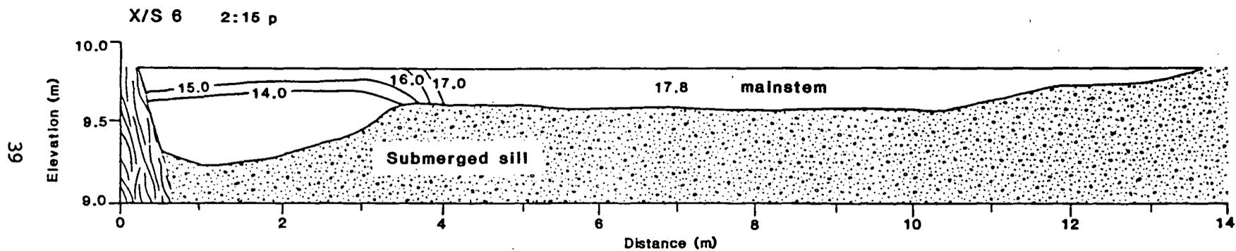
Figure 24. A temperature profile on the downstream end of the Elam Creek Cold Pool (Cross Section 6) shows that the submerged gravel bar sill and colder pool water effectively inhibits mixing of mainstem water with cold pool water.
