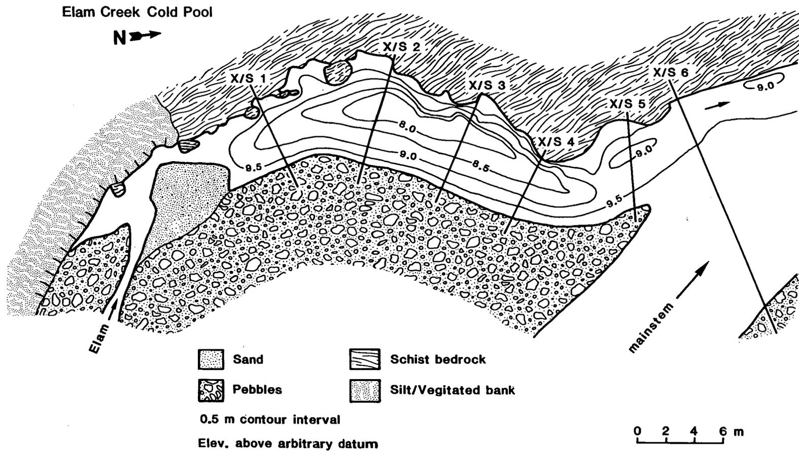
Figure 23. Topographic map of the Elam Creek Cold Pool showing cross section locations. This pool is located on the left side of the channel at the mouth of Elam Creek.
