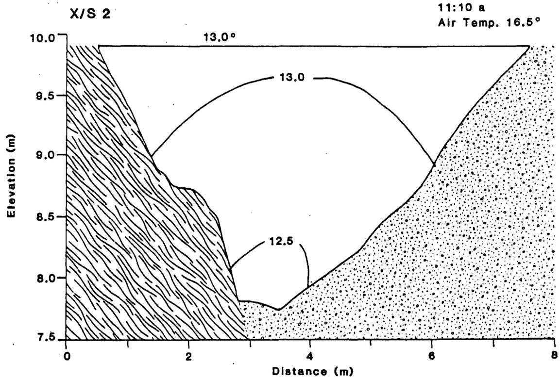
Figure 25. The temperature profile at Cross Section 2 in the Elam Creek Cold Pool shows that pool water was uniform in temperature.
