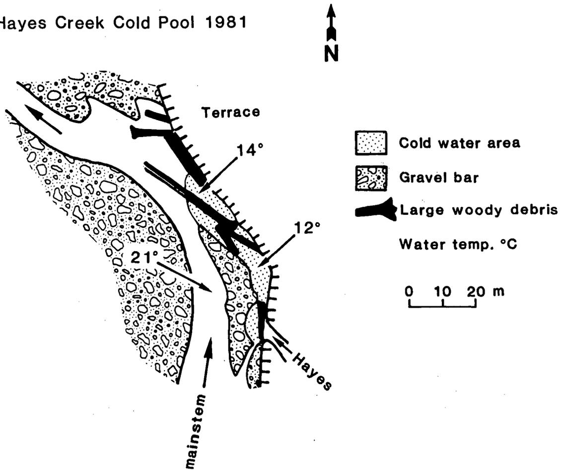
Figure 26. A cold pool developed at the mouth of Hayes Creek only when a gravel bar barrier separated the pool from the mainstem and concentrated cold water inflow (From Keller and Hofstra, 1983).
