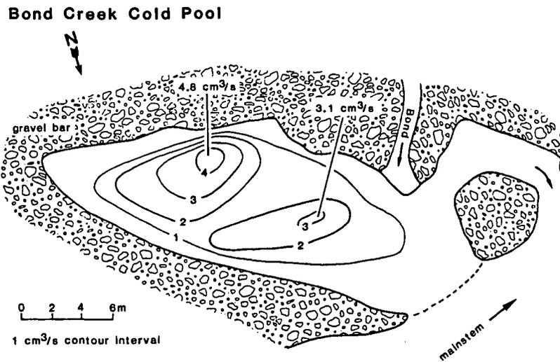
Figure 14. Seepage contour maps of Cold Pool A, Cold Pool B and the Bond Creek Cold Pool.
