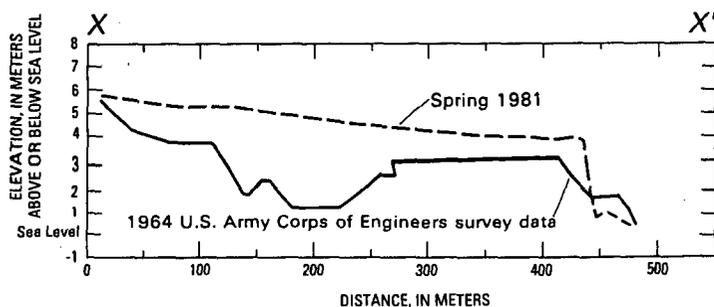
FIGURE 8.—Longitudinal dune profile X-X', mouth of Redwood Creek. Dune profile location is shown in figure 2.
