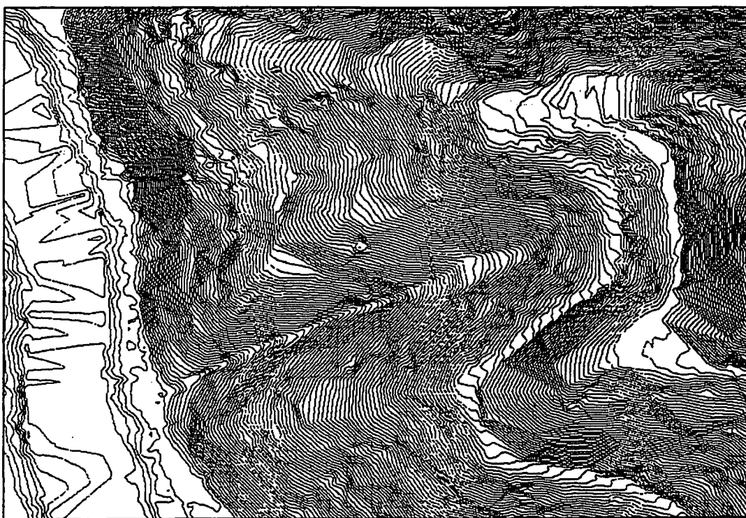
Figure 13. A portion of a one-meter contour interval map of the Scottsburg study area developed from a one-meter digital elevation model (DEM). This area is identical to that in Figure 11 & 12 (1 inch = 190 feet).
