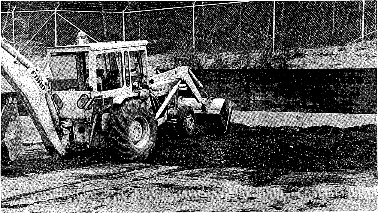
Figure 1: Bulking material is thoroughly mixed on the mixing pad and shaped into a saucer. All photographs are by the author and were taken in July 1982.
