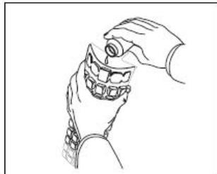
4. Pour the reagent/sample mixture directly into the Quanti-Tray avoiding contact with the foil tab. Allow foam to settle.
