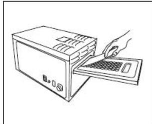
5. Place the sample-filled Quanti-Tray onto the rubber tray carrier of the Quanti-Tray Sealer with the well side (plastic) of the Quanti-Tray facing down to fit into the carrier.
