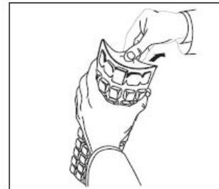
3. Open the Quanti-Tray by pulling the foil tab away from the well side. Avoid touching the inside of the foil or tray.
