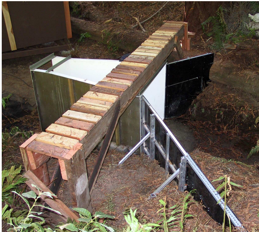
Figure 9--Montana Flume with wing walls and sampling bridge (the creek flows from right to left), Xray tributary, Caspar Creek Experimental Watershed, California.
