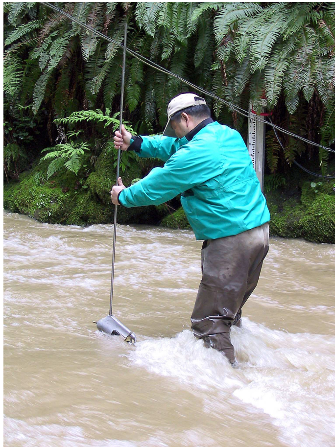
Figure 19--Collecting a suspended sediment sample using a US DH-48 wading type sampler.
