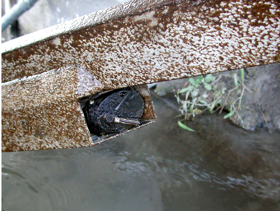
Figure 22--Optical contamination due to the wiper not being activated, Guadalupe River near San Jose, California.
