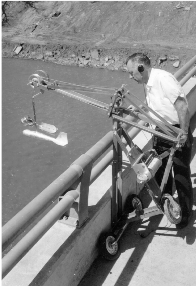
Figure 12--Discharge measurement from bridge using a crane, reel, and sounding weight. (Photo courtesy of the US Bureau of Reclamation).
