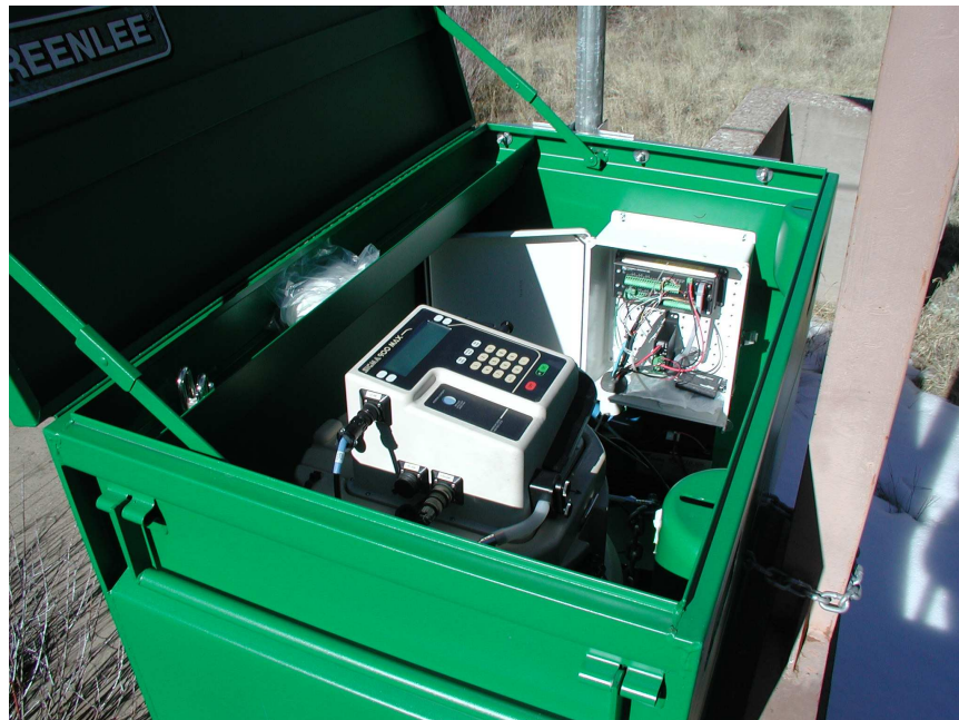
Figure 16--Lock box equipment shelter, Beaver Creek, Arizona. (Photo courtesy of the Arizona Department of Environmental Quality).
