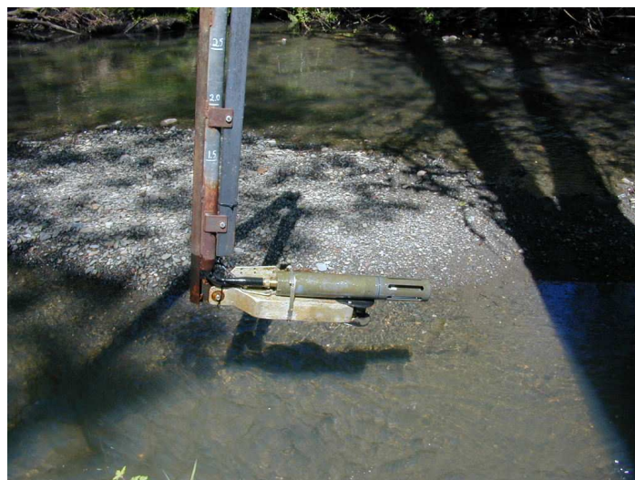
Figure 6--Deposition at Freshwater Creek, California, resulted in inadequate sampling depth at sensor location.
