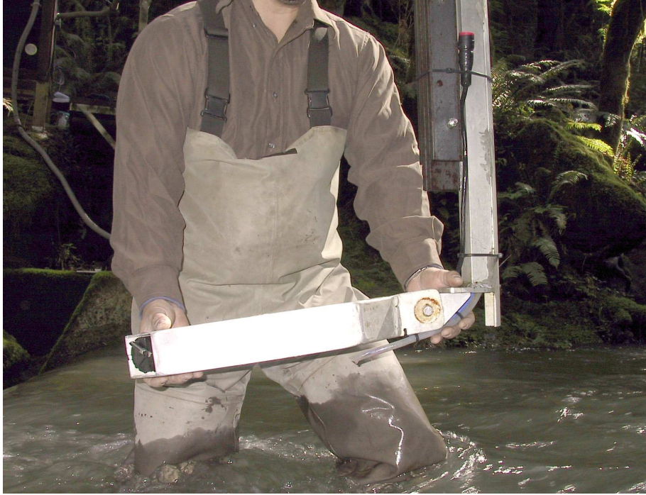
Figure 21--This housing for a DTS-12 sensor was constructed from square aluminum tubing, cut off diagonally at the optical end, which is oriented downstream.
