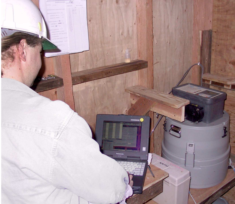
Figure 14--A walk-in shelter provides a dry environment for retrieving data and pumped samples and recording field notes.
