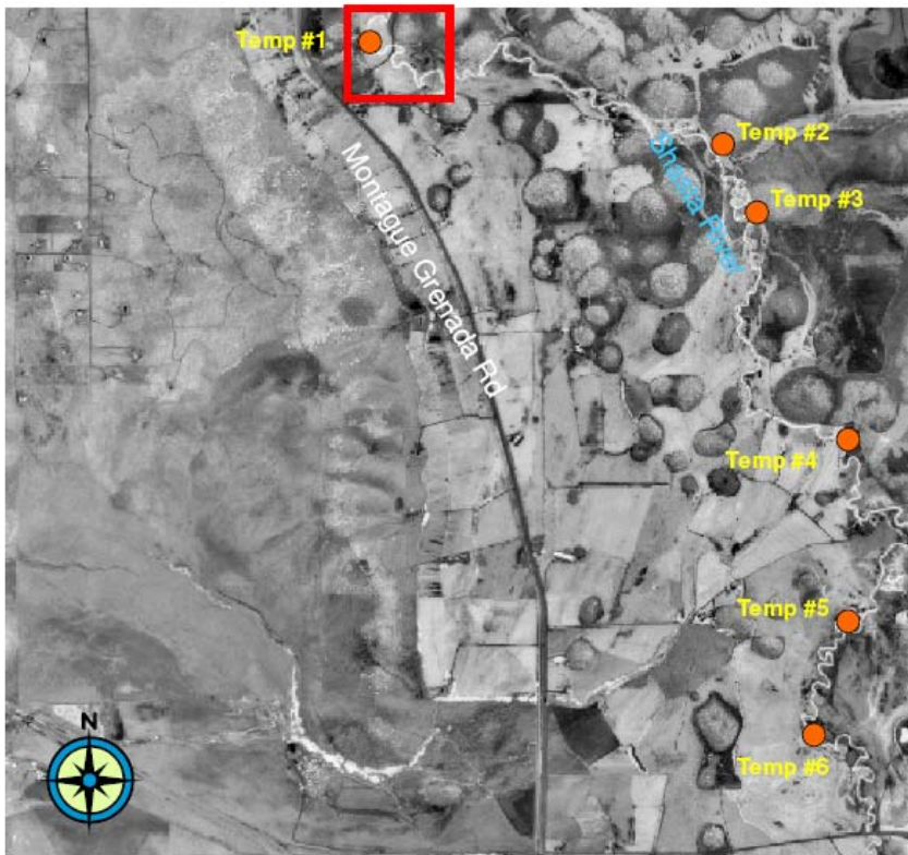
Figure 2: Planned locations for HOBO Temperature Probes- Shasta River Water Association.
