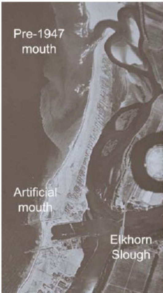
Figure 15 1946 aerial photo showing construction of new artificial Slough mouth in line with main channel, and smaller natural mouth to the north [ESNERR collection] (Elkhorn Slough, Website Report-1)
