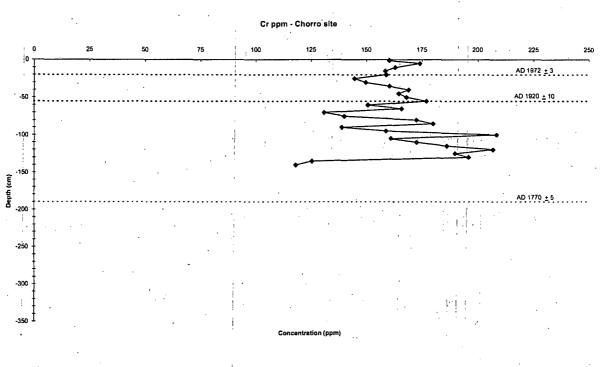
Figure 11: Sediment core of Chorro site (site A) indicating chromium concentration plotted against depth<sup>5</sup>.
