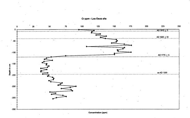
Figure 13: Sediment core of Los Osos site (site C) indicating chromium concentration plotted against depth.
