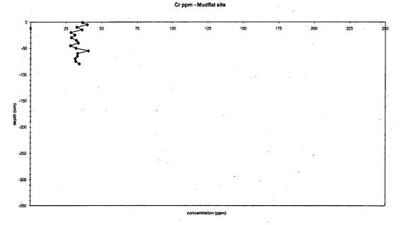
Figure 14: Sediment core of Mudflat site (site D) indicating chromium concentration plotted against depth<sup>6</sup>.
