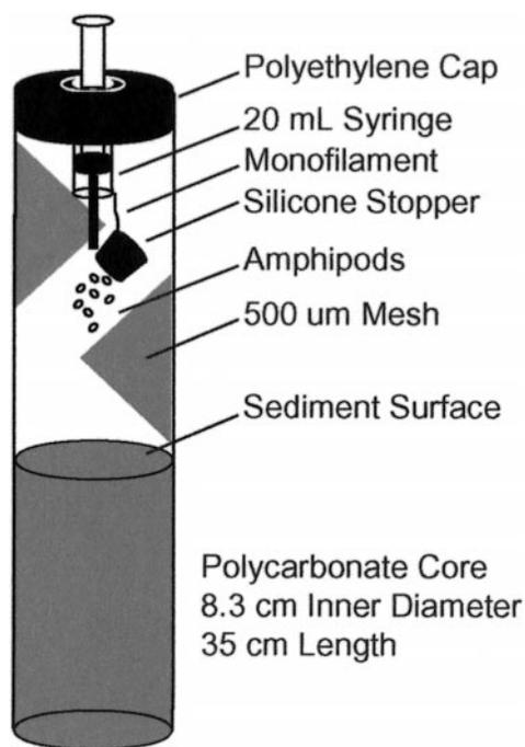
Fig. 3. Schematic of *Hyalella azteca* exposure tube.
