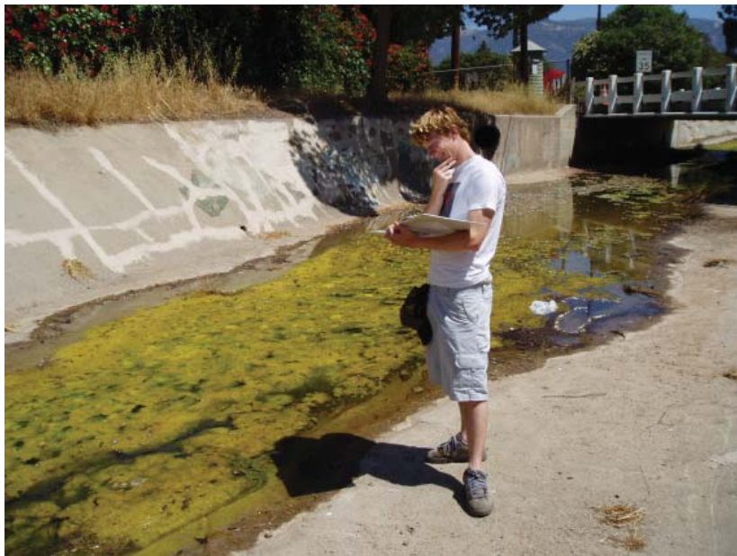
Site AT3, with warm, shallow flows in a wide concrete channel, is often choked with algae.
