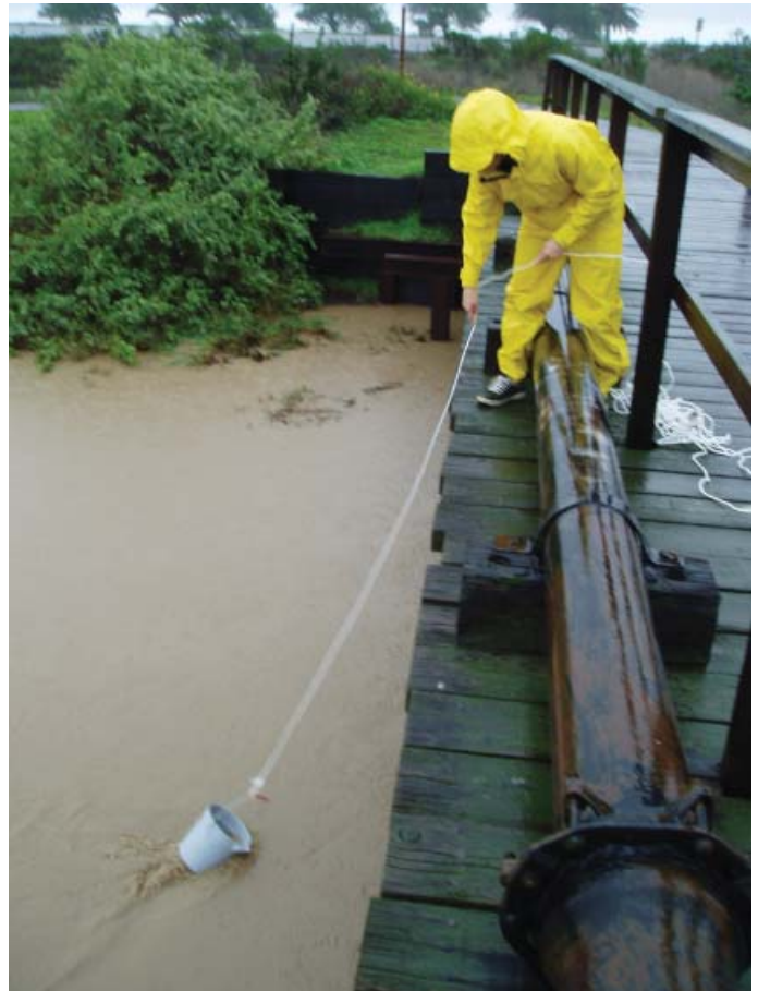
During the large storms of January 2005, sampling was conducted by lowering buckets from bridges.
