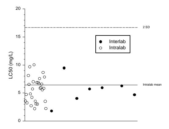
FIGURE B2. Cadmium reference toxicant median lethal concentrations (LC<sub>50</sub>) for the interlaboratory exercise (filled circles) and for a single laboratory (open circles).
