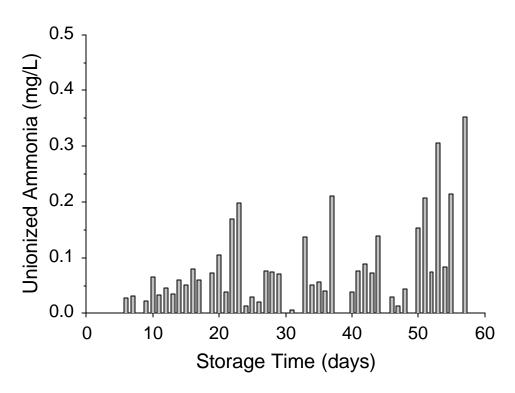
FIGURE III-3. Concentration of ammonia in elutriate samples stored prior to QwikSed analysis. Values are the mean of all samples stored for the indicated number of days.
