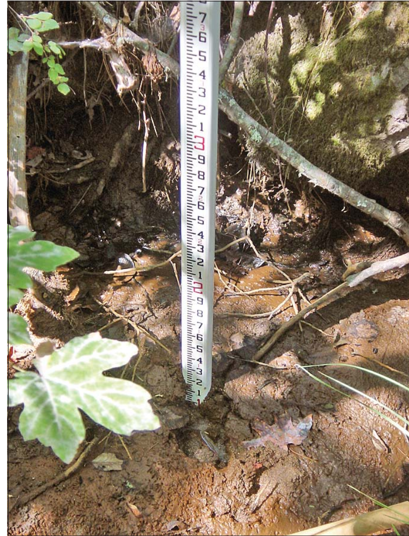
SCR-10. Close-up of silt and sand accumulation within channels; upstream of local obstructions.
