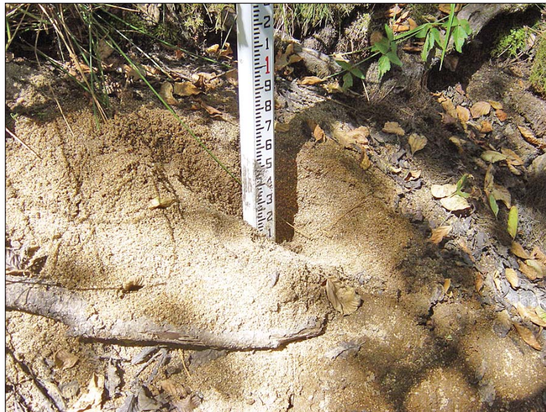
SCR-10 (the Outdoor School property). Close-up view of silt and sand (top) and sand and small gravel (bottom) accumulation within the channel (upstream of local obstructions). Such accumulations were fairly typical of the headwater streams draining the northern half of the upper Sullivan and Phoenix Lake watershed. The residence time of such sediments in the entire system is unclear, yet these are likely flushed out of local storage every year or so.
