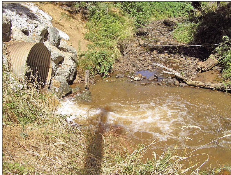
SCR-9. Looking upstream (top) from road, much more flow relative to other tributaries. Morphology appears to be plane-bed, or gentle cascade. Note the turbid nature of the water. Large culvert (bottom) is just upstream of reach in the top photo, it drains a tributary that comes in from the northwest and passes just to the west of the power station. The power station is likely using the water from the Penstock ditch (canal, etc.) and the effluent is diverted back into this tributary.
