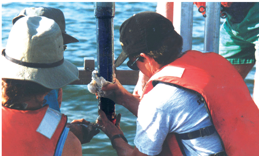
Collection of sediment cores from Hemet Lake. (photograph by Jennifer Wilson, U.S. Geological Survey)
