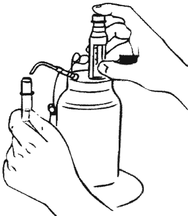
Figure 3. Adding 7.11M \text{H}_2\text{SO}_4 / 0.79M \text{MgCl}_2 Solution
