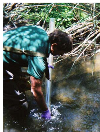
Figure 2-2. Collecting sediment samples by wading into the channel and manually pushing the core into the sediment.
