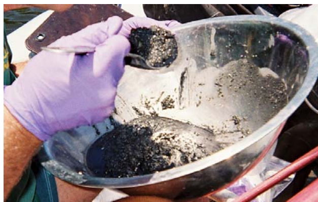
Figure 2-3. Composite being mixed in the field.
