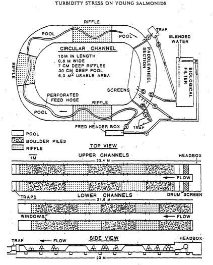
IGURE 1.—Generalized schematic of raceway channels at Hayden Creek Research Station and oval channels at University of Idaho showing the channel configurations, location of riffle and pool areas, and traps. (V = valve, D = drainline or drain, and P = pump.)
