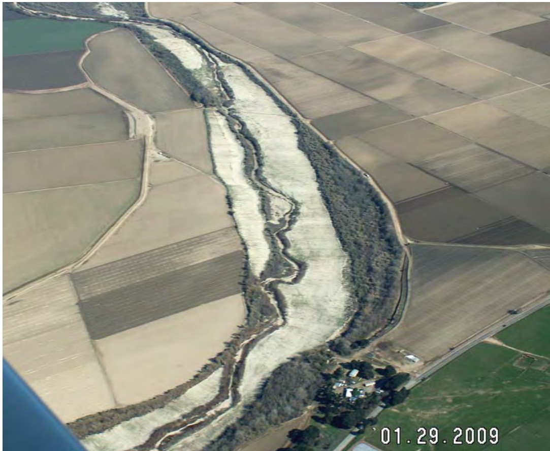
Figure 3. Aerial photo of the lower Salinas River in a typical reach below RM 23 where flood channel capacity can only accommodate an 8 year recurrence flood interval event (33,000 cfs). Note dwellings and agricultural operations in natural flood zone. Image provided by Steve Shimek of Monterey Coastkeeper.
