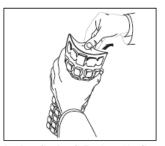
Open the Quanti-Tray by pulling the foil tab away from the well side. Avoid touching the inside of the foil or tray.
