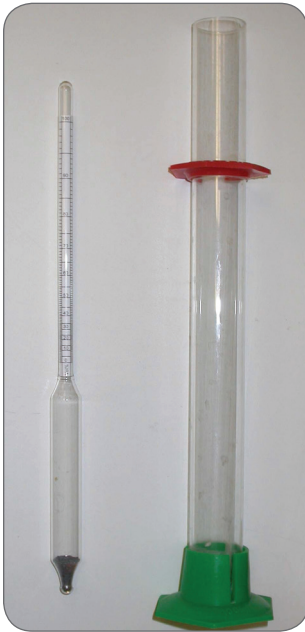
Figure 1: Hydrometer and 150 mL graduated cylinder used to check sample preservation levels.
