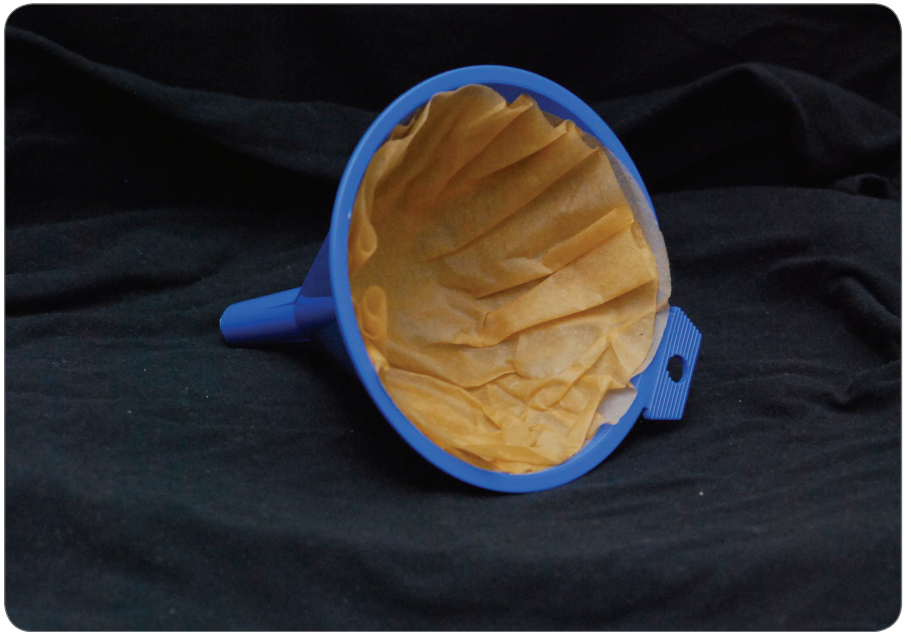
Figure 2: Example of filtered funnel used to keep particulates out of the waste stream.
