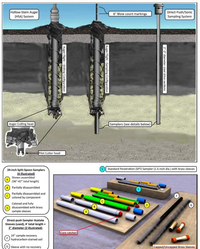
Figure 15-1: Common Drilling Methods and Soil Sampling Systems
