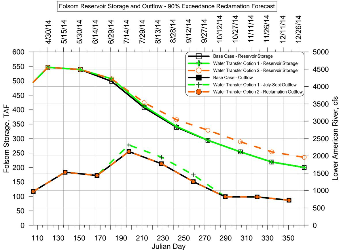
Figure 2. Folsom Reservoir Storage and Lower American River Flow for the Base Case and for the Alternative Water Transfer Release Options 1 and 2.
