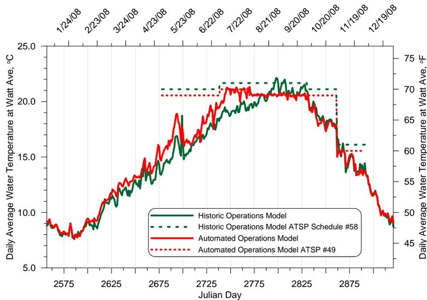
**Appendix C Figure 9. Comparison of Historical Versus Automated Model Operations for Watt Avenue Water Temperature, 2008. (Note: These results were obtained by using a combination of the CE-QUAL-W2 model and an American River water temperature regression between Folsom Dam and Watt Avenue).**
