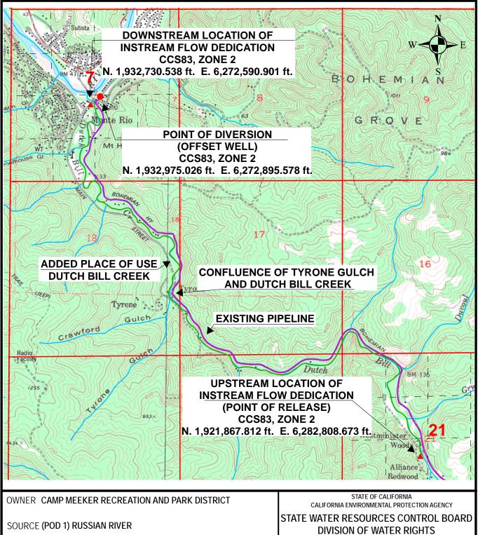
POINT OF DIVERSION APPLICATION NO. 31055 PERMIT NO. 21198 WITHIN NW 1/4 OF SE 1/4 OF PROJECTED **URGENCY CHANGE** SECTION 7, T7N, R10W, MDB&M COUNTY OF SONOMA CHECKED: U.S.G.S. QUAD: DUNCAN MILLS DATE: PH. RE. 1981 SCALE: 1:25,000 9-2-2015 Note: This map does not constitute a public land survey as defined by California Business & Professions Code section 8726. It has been prepared for descriptive purposes only.
