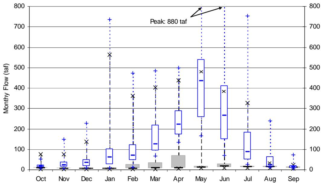
Key to boxplots: Median, horizontal line; box, 25th and 75th percentiles; whiskers, range for unimpaired flow (“+” sign) and observed (“x” sign).
