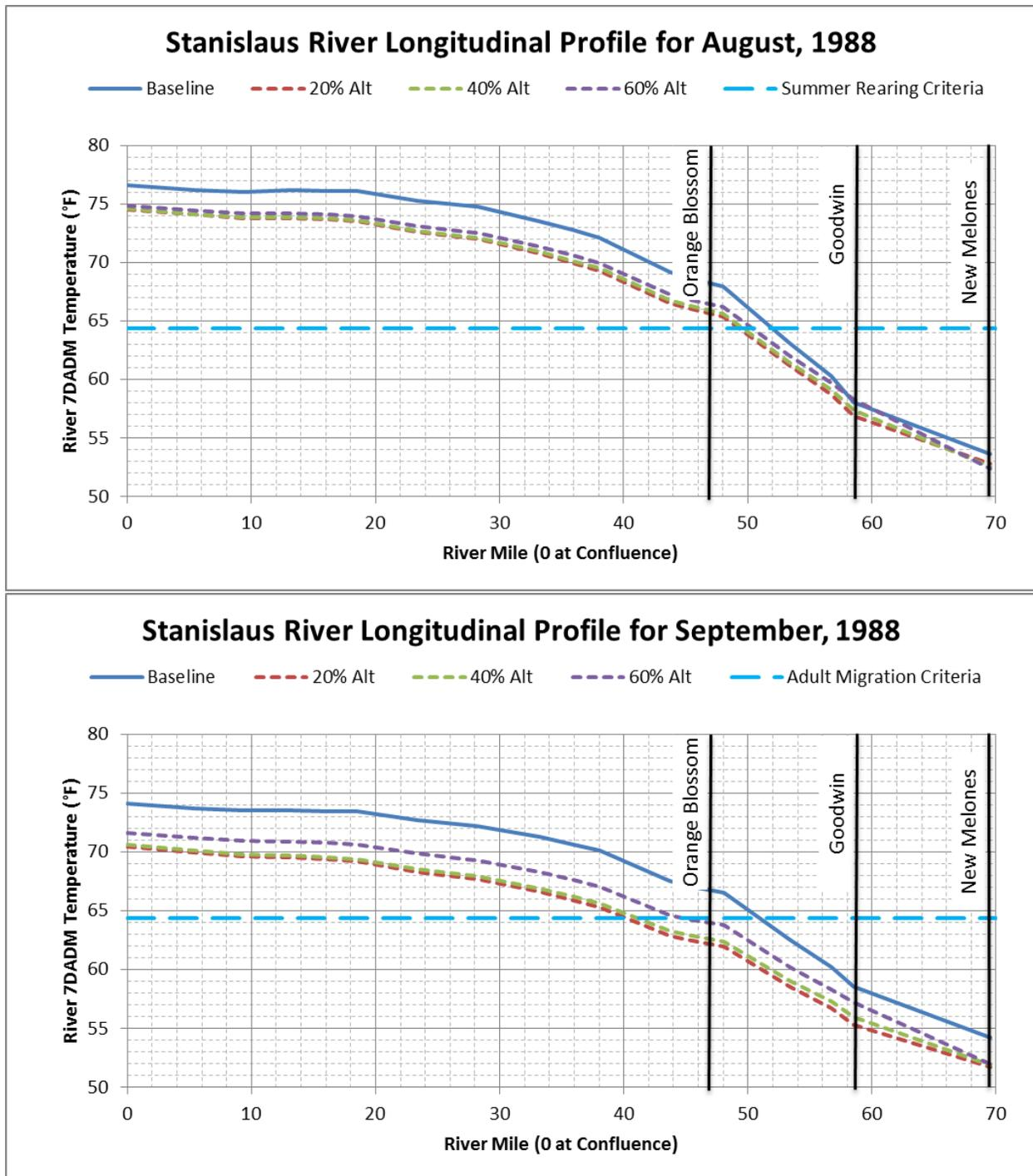
**Figure F.1.6-19. Longitudinal Monthly Average 7DADM Temperature Results within the Stanislaus River for (a) August 1988 and (b) September 1988**
