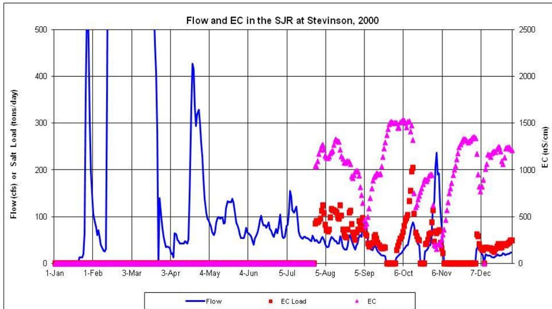
**Figure F.2-2a. Daily Measured Flow (cfs) and EC ( $\mu\text{S}/\text{cm}$ ) and Calculated Salt Load (tons/day) in the SJR at Stevinson during 2000**
