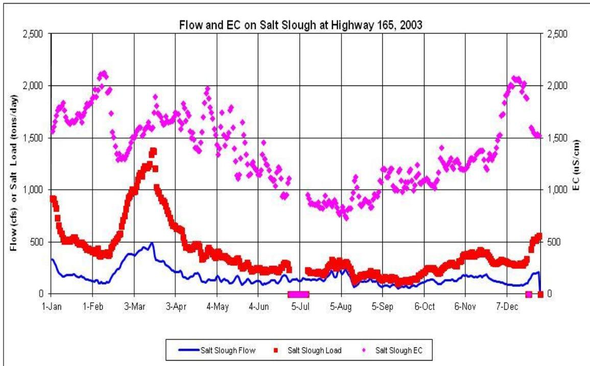
**Figure F.2-5b. Daily Measured Flow (cfs) and EC ( $\mu\text{S}/\text{cm}$ ) and Calculated Salt Load (tons/day) in Salt Slough at Highway 165 during 2003**
