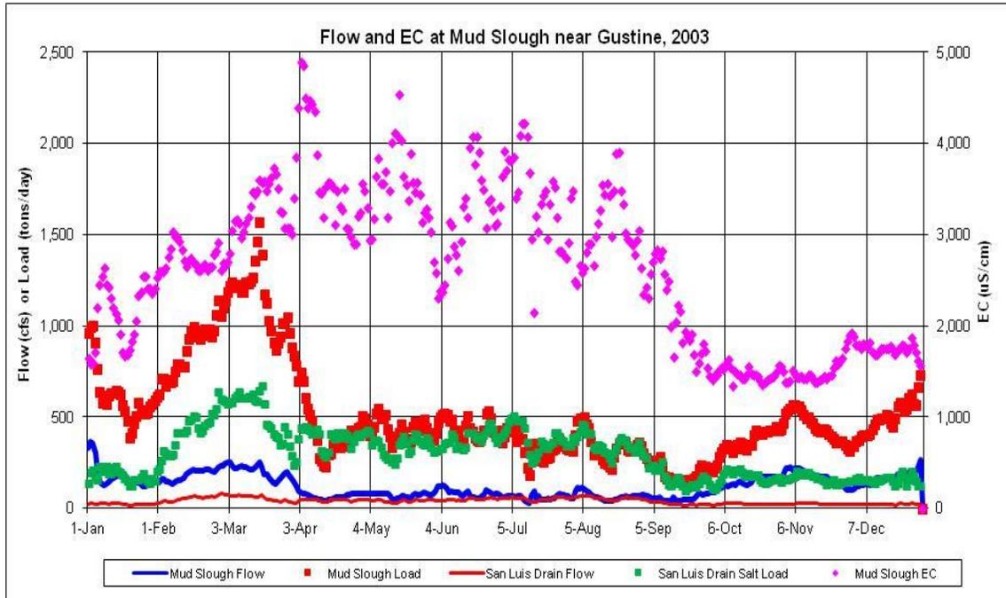
**Figure F.2-5c. Daily Measured Flow (cfs) and EC ( $\mu\text{S}/\text{cm}$ ) and Calculated Salt Load (tons/day) in Mud Slough near Gustine and in the San Luis Drain Discharge to Mud Slough during 2003**
