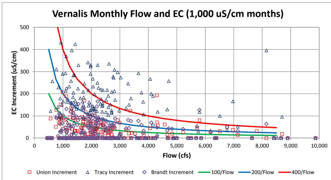
**Figure F.2-11b. Monthly Average Vernalis Flow and Monthly Average EC Increments from Vernalis to Brandt Bridge, Union Island and Tracy Bridge for September–March (1,000  $\mu\text{S}/\text{cm}$  EC objective) of WY 1985–2010**
