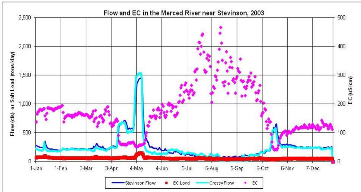
**Figure F.2-5d. Daily Measured Flow (cfs) and EC ( $\mu\text{S}/\text{cm}$ ) and Calculated Salt Load (tons/day) in the Merced River near Stevinson during 2003**
