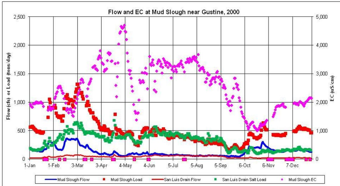
**Figure F.2-2c. Daily Measured Flow (cfs) and EC ( $\mu\text{S}/\text{cm}$ ) and Calculated Salt Load (tons/day) in Mud Slough near Gustine and in the San Luis Drain Discharge to Mud Slough during 2000**
