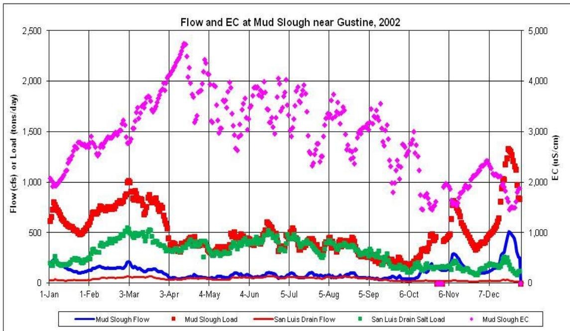
**Figure F.2-4c. Daily Measured Flow (cfs) and EC ( $\mu\text{S}/\text{cm}$ ) and Calculated Salt Load (tons/day) in Mud Slough near Gustine and in the San Luis Drain Discharge to Mud Slough during 2002**
