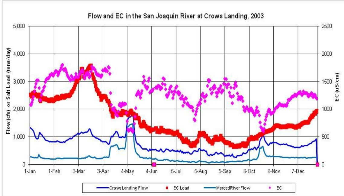
**Figure F.2-5e. Daily Measured Flow (cfs) and EC ( $\mu\text{S}/\text{cm}$ ) and Calculated Salt Load (tons/day) in the SJR at Crows Landing (downstream of the Merced River) during 2003**
