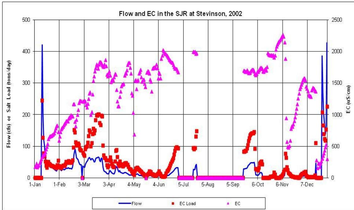
**Figure F.2-4a. Daily Measured Flow (cfs) and EC ( $\mu\text{S}/\text{cm}$ ) and Calculated Salt Load (tons/day) in the SJR at Stevinson during 2002**
