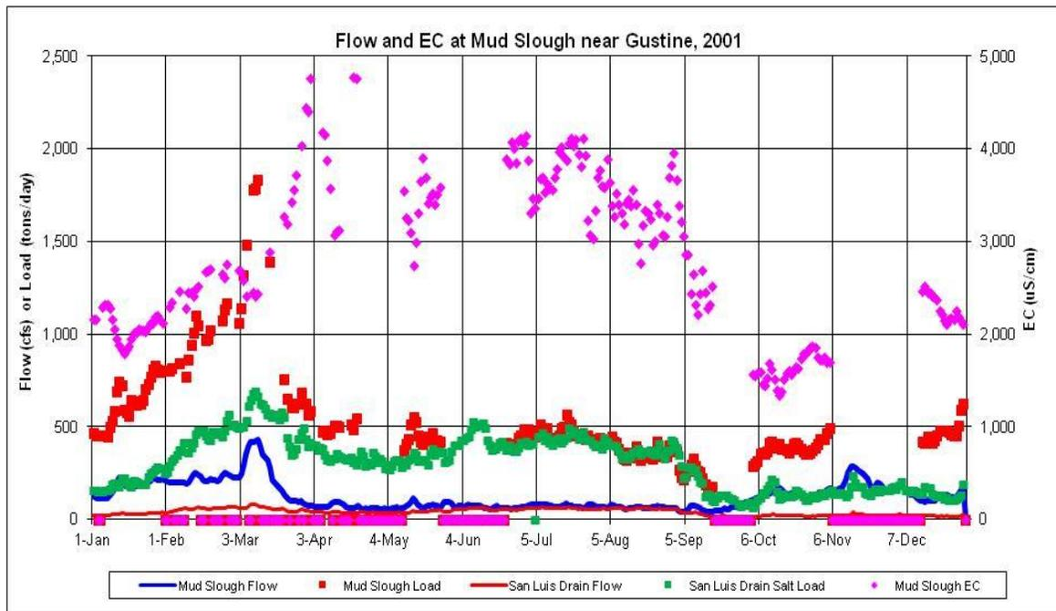
**Figure F.2-3c. Daily Measured Flow (cfs) and EC ( $\mu\text{S}/\text{cm}$ ) and Calculated Salt Load (tons/day) in Mud Slough near Gustine and in the San Luis Drain Discharge to Mud Slough during 2001**
