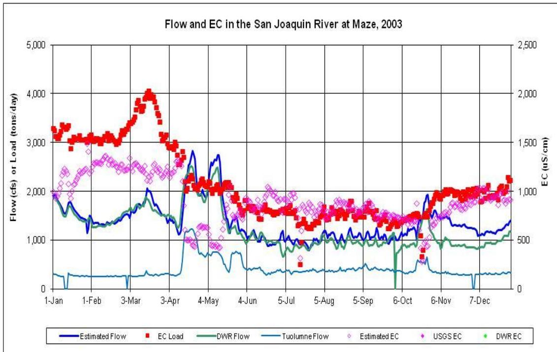
**Figure F.2-5f. Daily Measured Flow (cfs) and EC ( $\mu\text{S}/\text{cm}$ ) and Calculated Salt Load (tons/day) in the SJR at Maze (downstream of the Tuolumne River) during 2003**
