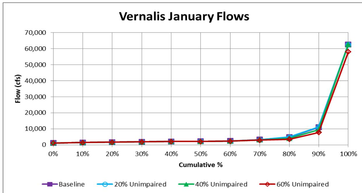
**Figure F.1.4-4m. WSE-Simulated Cumulative Distributions of SJR at Vernalis January Flows (cfs) for Baseline Conditions and 20%, 40%, 60% Unimpaired Flow (LSJR Alternatives 2–4)**
