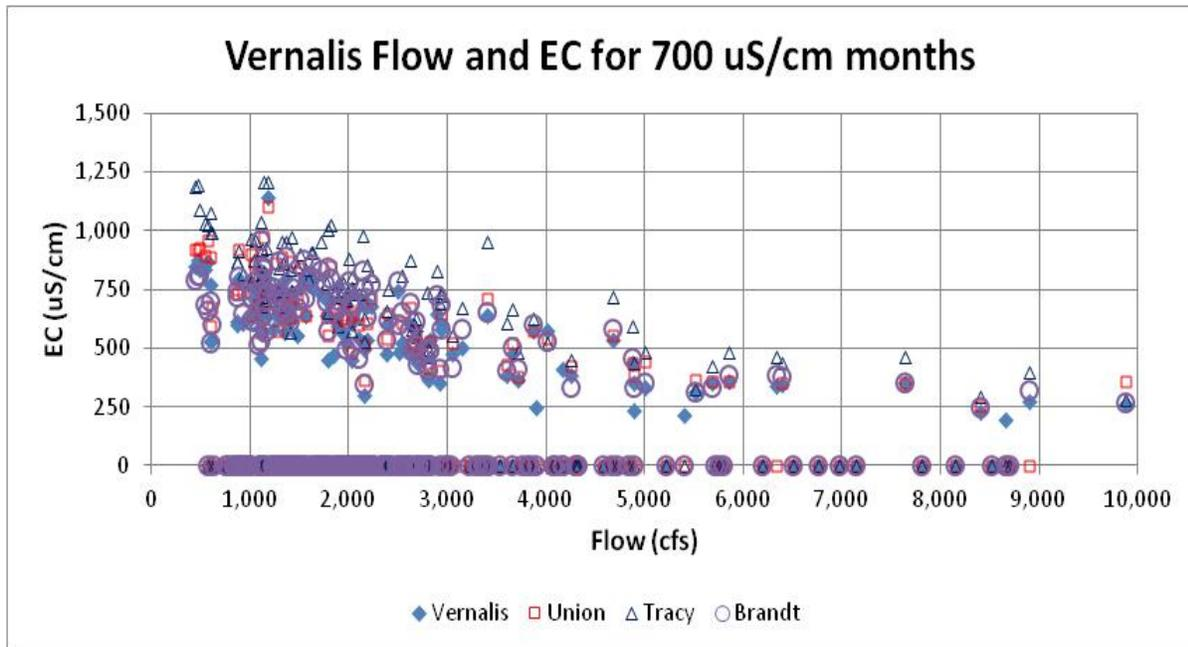
Figure F.2-10a. Monthly Average Vernalis Flow and Monthly Average Measured EC at Vernalis, Brandt Bridge, Union Island and Tracy Boulevard for April–August (700  $\mu\text{S}/\text{cm}$  EC objective) of WY 1985–2010
