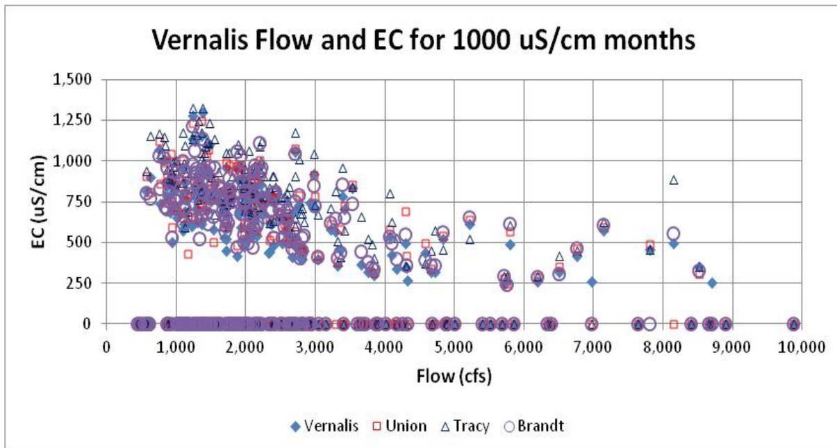
Figure F.2-10b. Monthly Average Vernalis Flow and Monthly Average Measured EC at Vernalis, Brandt Bridge, Union Island and Tracy Boulevard for September–March (1,000  $\mu\text{S}/\text{cm}$  EC objective) of WY 1985–2010
