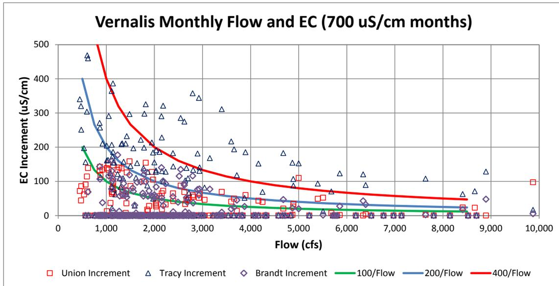
**Figure F.2-11a. Monthly Average Vernalis Flow and Monthly Average EC Increments from Vernalis to Brandt Bridge, Union Island and Tracy Bridge for April–August (700  $\mu\text{S}/\text{cm}$  EC objective) of WY 1985–2010**
