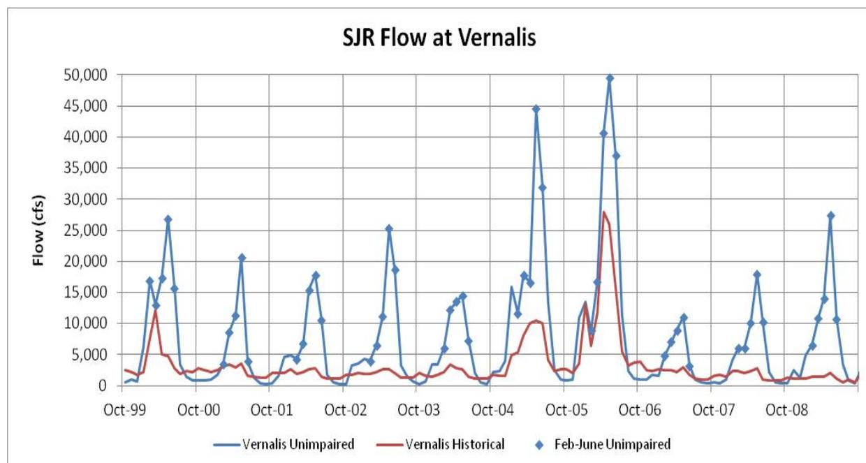
**Figure 2-11. Monthly Unimpaired and Historical LSJR Flows at Vernalis February–June for Water Years 2000–2009 (cfs = cubic feet per second)**
