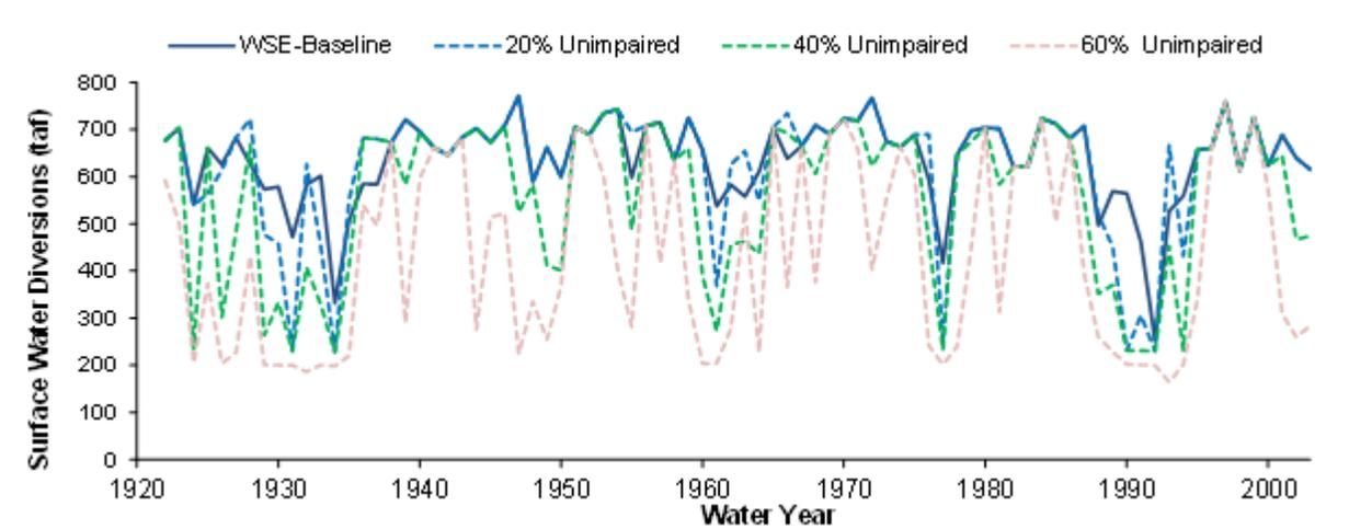
**Figure 2.3-5. Comparison of WSE Model Results for Baseline and LSJR Alternatives: Stanislaus River Diversions for 1922–2003 (taf = thousand acre-feet) (Copy of Figure 5-9 of Chapter 5)**
