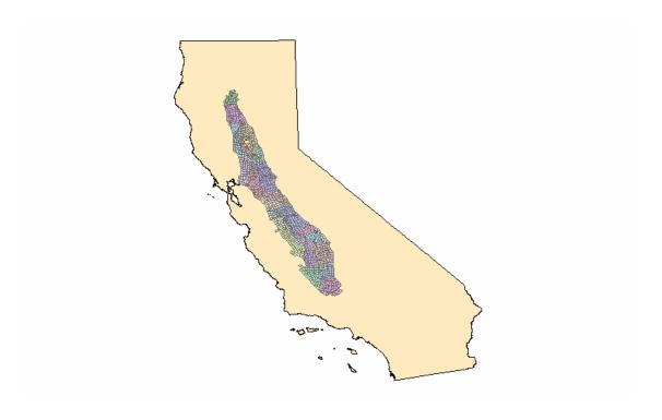
Figure F-2 CVGSM2 Finite Element Grid and Subregions
