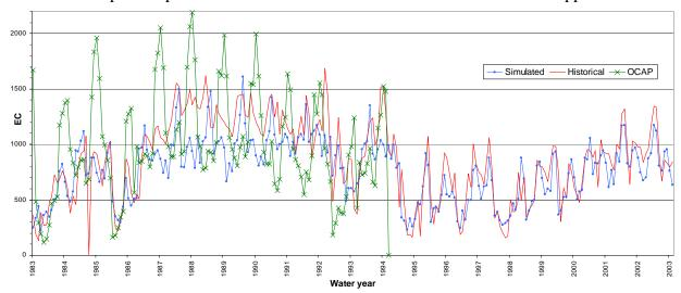
Figure 14. New (Simulated) and Old (OCAP) Model Results and Historical Data for Maze EC (μS/cm) since 1983 (OCAP ends with 1994)
