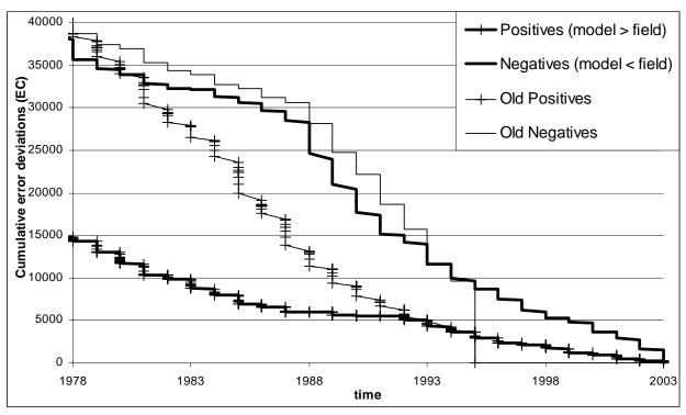
Figure B2. Cumulative positive and negative deviations of new and old CalSim II models from historical data, going backwards from 2003. Old model results (which end in 1994) are begun at the same values as the new model in 1994.
