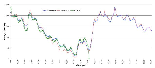
Figure 7. Historical Data and New (Simulated) and Old (OCAP) Model Results for New Melones Storage (OCAP ends with 1994)
