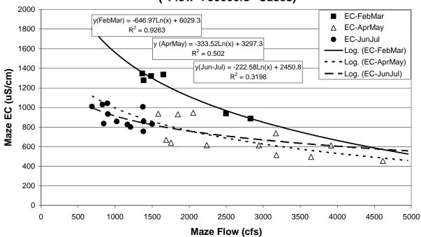
Figure B5. Flow versus (µS/cm) data for Maze
