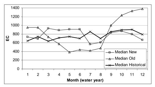
Figure 15. Median Monthly Maze EC (µS/cm), 1940-2003 (old model to 1994)
