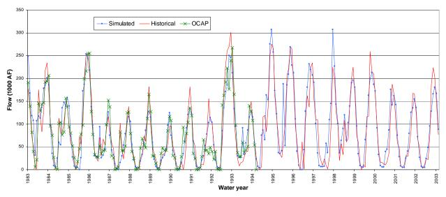
Figure 2. Historical Data and New (Simulated) and Old (OCAP) Model Results for Friant-Kern Canal Diversions (OCAP ends with 1994)
