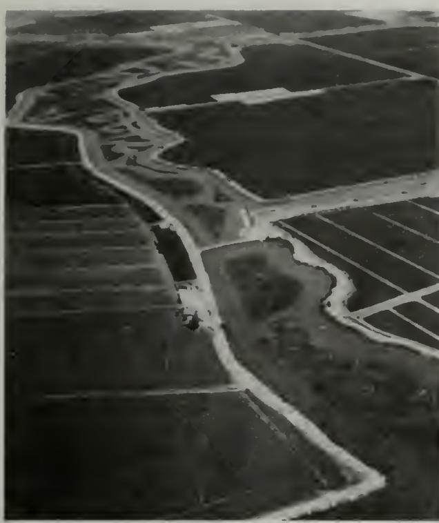
*Disappointment Slough looking west near where the Peripheral Canal will cross. The first stage of the canal, which will be siphoned under the slough, will terminate just south of here. Water from the Peripheral Canal will be released into Disappointment Slough and other sloughs along the canal route to improve the water quality.*
