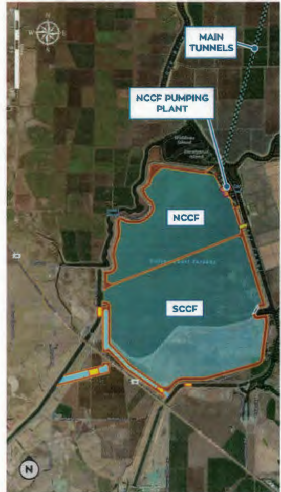
Figure 6: Clifton Court Forebay, including proposed modifications
