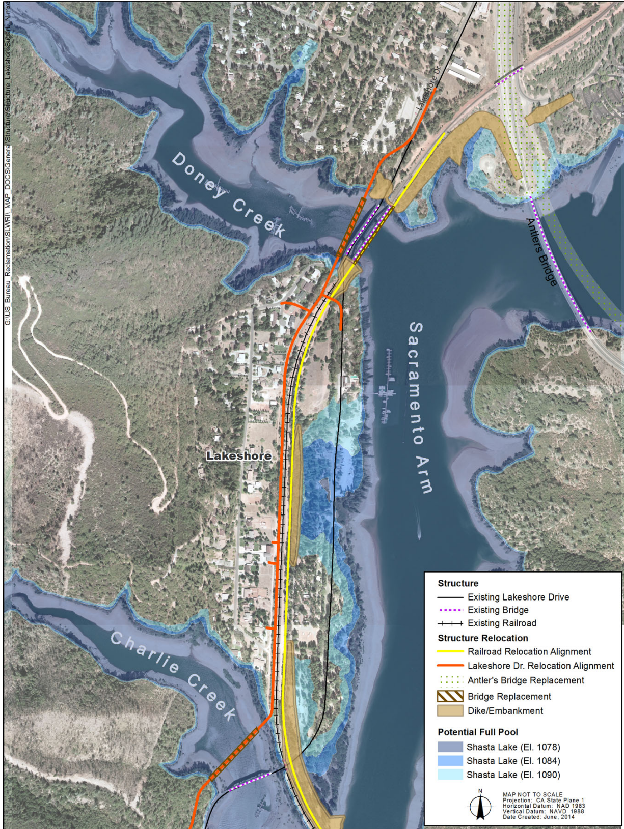
Figure 4-5. Estimated Maximum Inundation in the Lakeshore Area for 6.5-foot, 12.5-foot, and 18.5-foot Dam Raises
