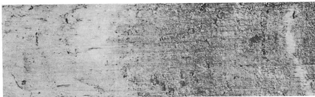
Figure 2. (–5.0 to 5.5 feet) Irregularly laminated, root-riddled, inorganic flood-basin silty clay; barren of fauna.
