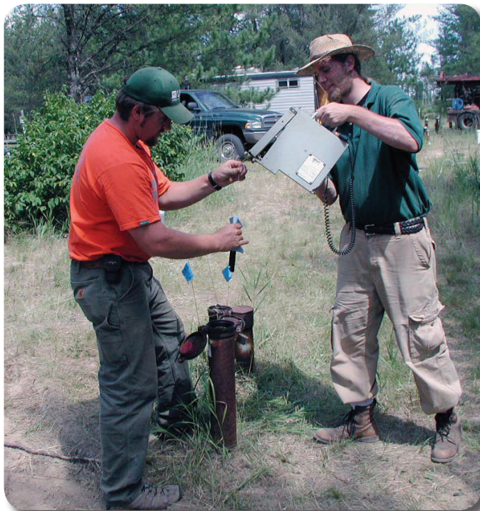
Bemidji Crude-Oil Research Project; measuring crude-oil thicknesses during the aquifer test.
