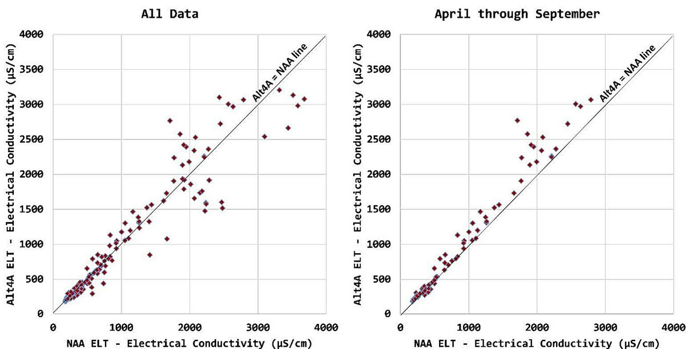
**Figure 4. Scatter Plot Showing Average Monthly EC Values between Alt4A ELT and NAA ELT in the Sacramento River at Three Mile Slough**
