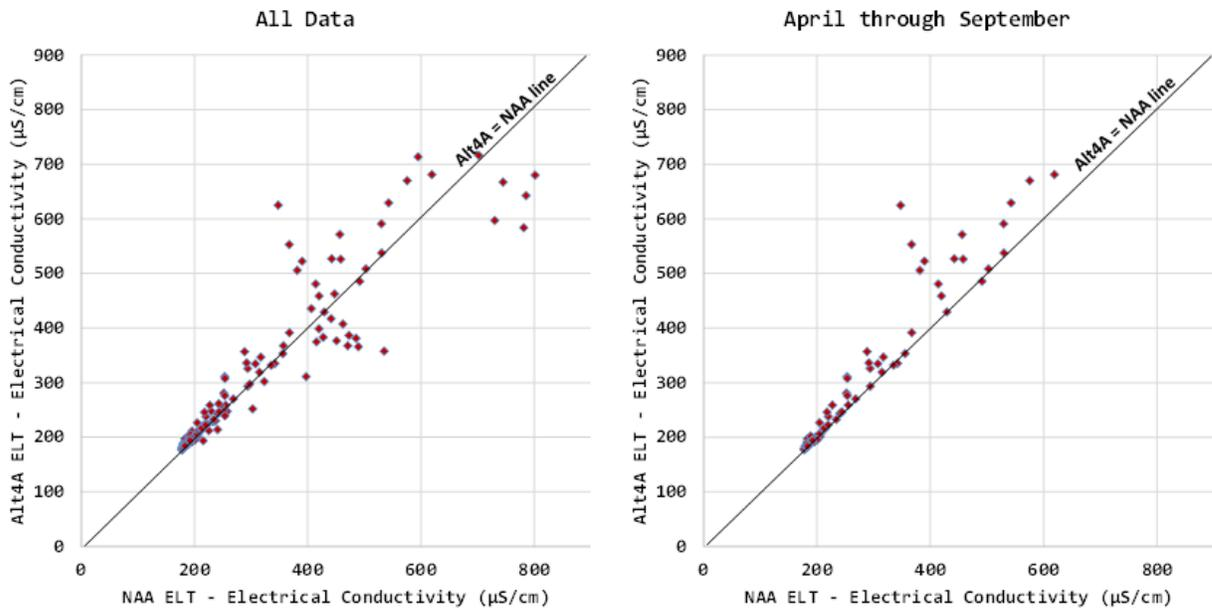
Figure 6. Scatter Plot Showing Average Monthly EC Values between Alt4A ELT and NAA ELT in the Sacramento River at Rio Vista
