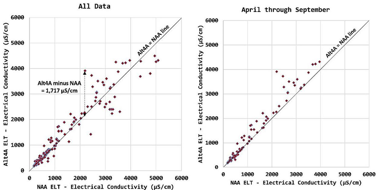
**Figure 2. Scatter Plot Showing Average Monthly EC Values between Alt4A ELT and NAA ELT in the Sacramento River at Emmaton**
