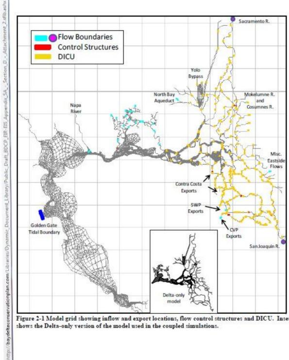
Figure 2-1 Model grid showing inflow and export locations, flow control structures and DICU. Inset shows the Delta-only version of the model used in the coupled simulations.
