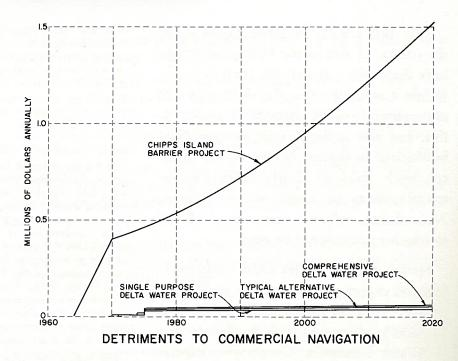
Construction of control structures and closures on channels south of the San Joaquin River in the heart of the Delta would increase time and distance for tug and barge travel to a sugar refinery near Tracy. However, channel improvements would permit use of larger barges, if shipping concerns should elect to do so. As this advantage would be subject to many factors in an operator's business which cannot be readily predicted, benefits were not claimed for possible use of larger barges.
