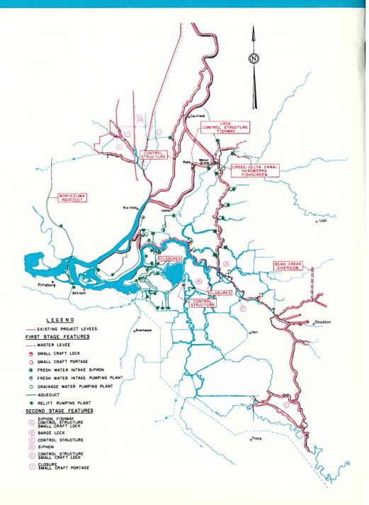
About 1,900 acres of Delta land would be filled with excess dredged material, and most of this land would be available for recreational development. The additional gates on the Cross-Delta Canal headworks and the extensions of the adjacent highway and railroad bridges would be constructed with about 16 feet of clearance above the present average water level to improve small craft access between the Sacramento River and channels of the Mokelumne River system.
