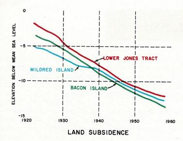
underlying sand aquifers will be reduced. Unless suitable methods of arresting the loss of peat are developed, farming in the Delta will cause continued subsidence. Experience has shown that this subsidence will continue to within about two to three feet above the bottom of the peat. Significant tracts of Delta land will become impractical to farm unless seepage is controlled and the danger of inundation is reduced.
