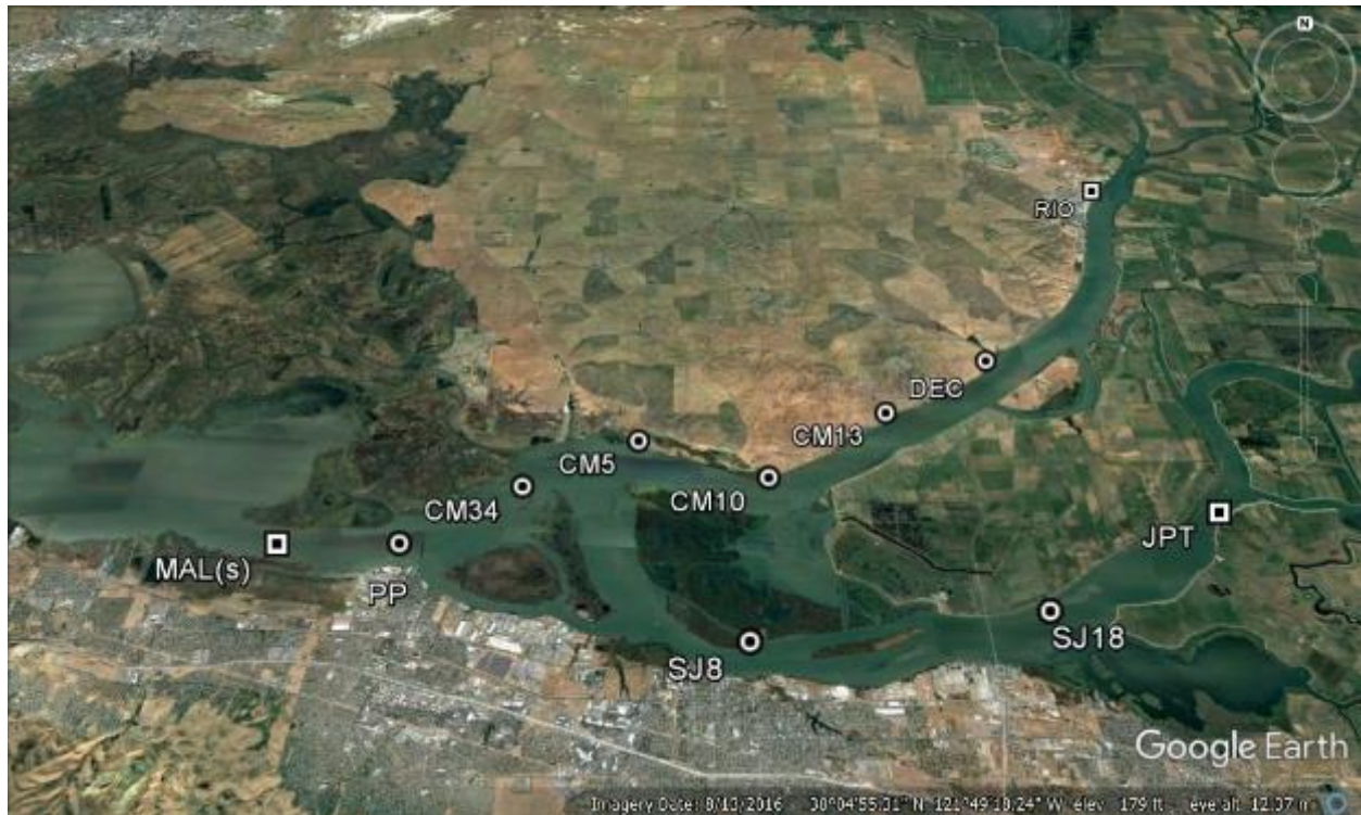
Figure 5-2 USGS Locations of Proposed Temperature, Salinity and Turbidity Monitoring Equipment. All of the stations proposed are new (circle icons), except at MAL(s), RIO and JPT (square icons), which are long-term monitoring stations run by the DWR-RTM.
