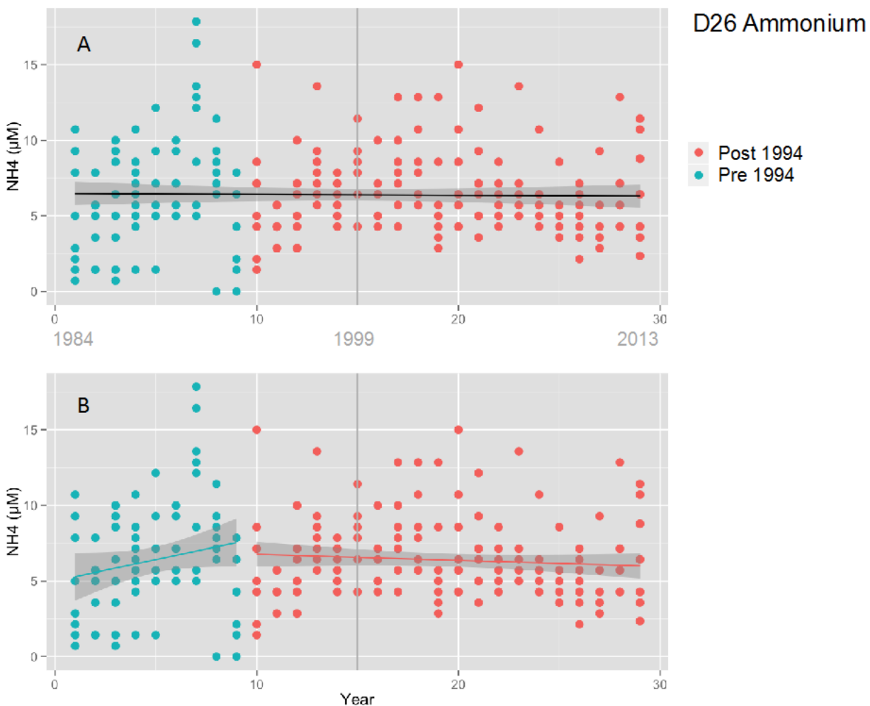
Figure A-2. Changes in the concentration of ammonium ( \text{NH}_4^+ ) over time (1985-2013) at station D26 in the Delta. Green filled circles denote period before 1994 and red filled circles denote the period after 1994. Vertical grey line denotes the year 1999 when Microcystis started occurring. A) Regression of \text{NH}_4^+ versus time for the period 1985-2013 (black line) with 95% confidence interval in grey. B) Regression of \text{NH}_4^+ versus time for the period 1985-1994 (green line) and the period 1994-2013 (red line). Slopes significantly different from zero in bold in regression table:
