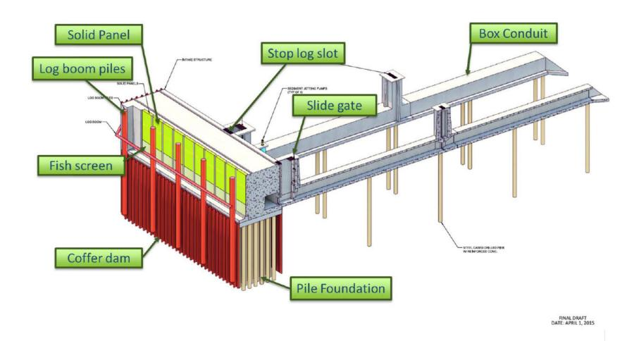
Figure 4- Isometric View of an Intake Bay
