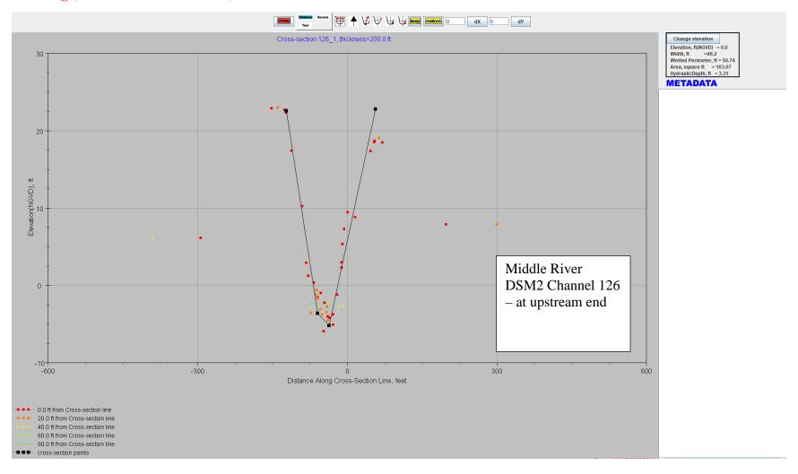
$DWR-1402-Example\ Middle\ River\ channel\ cross-sections\ in\ DSM2\ from\ 2009\ calibration,\ which\ is\ the\ basis\ for\ CWF\ modeling\ (Elevations\ in\ ft\ NGVD29)$
